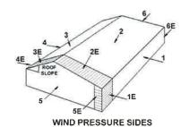
Load Case A: Winds generally perpendicular to ridge Load Case B. Winds generally parallel to ridge
