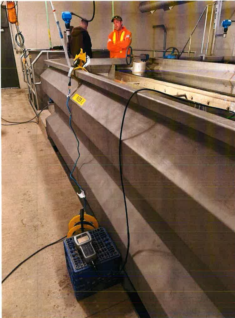
Picture 1. Filter #2 Turbidity testing on filter backwash
